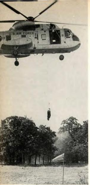
Dummy is hauled aloft during simulated rescue. Powerful downwash from blades stands windsock straight out.
